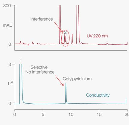
Figure 17. Selective detection of the cationic surfactant in mouthwash with SCD
