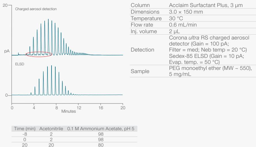
Figure 9. Sensitivity comparison of charged aerosol detection vs. ELS
